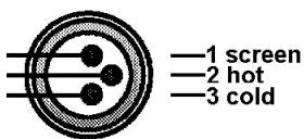
Both amplifier channels feature a balanced XLR female socket as well as a balanced 6.35 phone jack socket.
