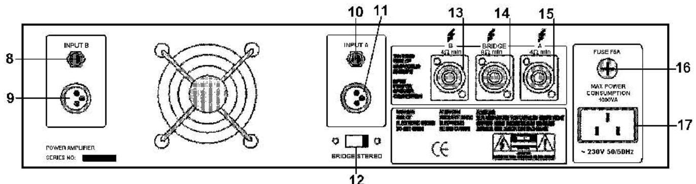
8. Channel B input through 6.35mm balanced mono jack.
