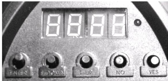
After powering on the device the display shows the DMX start address. Set the desired start address by means of the YES/NO buttons to increase or decrease the address. Press the ENTER button to confirm. The display will show “PASS” to confirm your settings. Other functions can also be selected by means of F-DOWN and F-UP buttons, changed by means of the NO, YES buttons and confirmed by means of the ENTER button.
