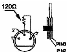
A DMX terminator is recommended for installations where the DMX cable has to run a long distance or is in an electrically noisy environment (e.g. discos). The terminator prevents corruption of the digital control signal by electrical noise. The DMX terminator is simply an XLR plug with a 120Ω resistor between pins 2 and 3, which is then plugged into the XLR output socket of the last device in the chain. Refer to the illustrations on the left.
