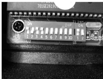
Set the DIP switches of the master device as follows. Choose an address from the table above.
