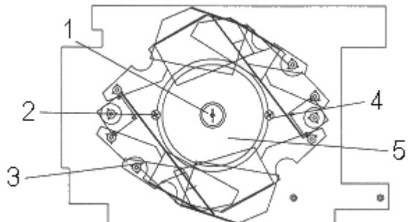
Carefully move the mirrors to the two sides so as to uncover the lamp. Use a Phillips-head screwdriver and carefully loosen the two screws in order to remove the reflector. Removing the reflector will uncover the lamp socket.
