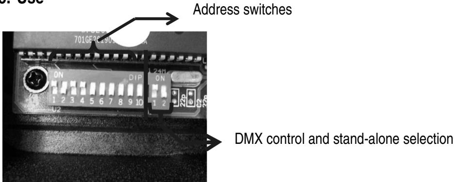
Set an address for stand-alone mode using DIP switches 1 to 10. See table below.
