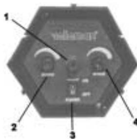
Connect the device with the mains through the power plug. Normally speaking it is not a good idea to connect lighting effects with dimming packs. Place the power switch (3) in the ON position. Adjust the music sensitivity with rotary control (2) and adjust the running speed with rotary control (4). The device will start to produce colourful light flashes to the rhythm of the music via the built-in microphone.
