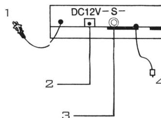
Connect the device to the mains via the AC power socket or use an optional AC/DC adapter. Plug the antenna plug (4) into the TV set.
