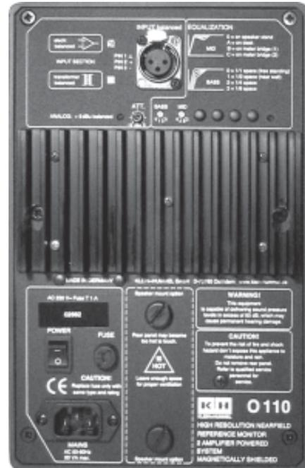
Figure 2: Rear panel of the O 110
