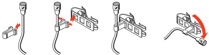
For thin clothes (e.g. silk), please use the outer hole where the clip's contact pressure is the highest.
