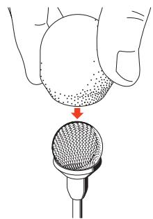
You may further reduce the wind noise by 10 dB by means of the additional MZW 02 foam-net wind-shield.
