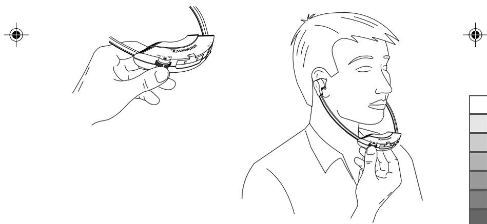
Use the rotary switch to switch on the receiver and adjust the volume.
