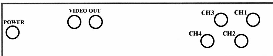
**BNC CONNECTORS (CH1-CH4) :** video signal input connections
